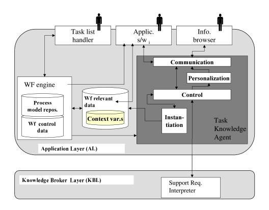
Figure 25: Generic Architecture for Application Layer
